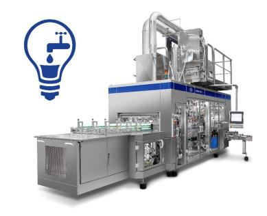
third generation filling machines for small and medium size carton packs can also be fitted with a newly developed, and easy-to-fit, water reduction conversion kit, which halves water consumption by saving approximately up to 350 litres per hour.
