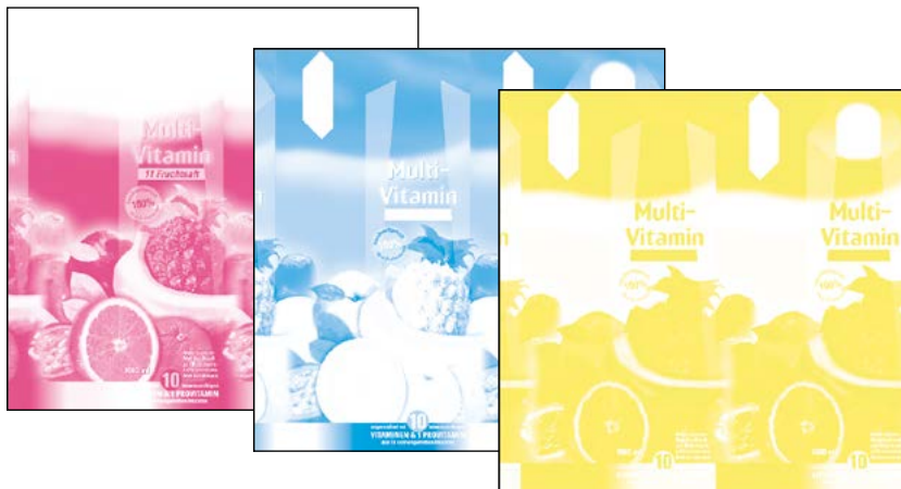
SIG standard printing with 3-colour build-up of the picture design
