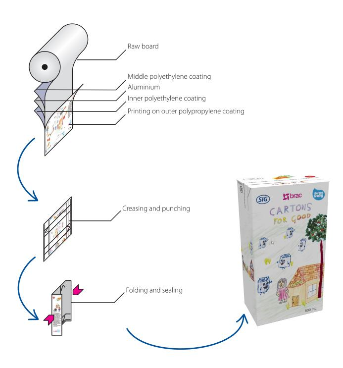
The preformed carton sleeves are produced in the packaging material facilities at SIG and they are later aseptically filled on the filling machines on the customer's premises. The carton is given an inside layer of high-grade polyethylene (PE) and an outside layer of high grade polypropylene (PP) layer including an extremely thin layer of aluminium and another inner layer of polyethylene (PE).
