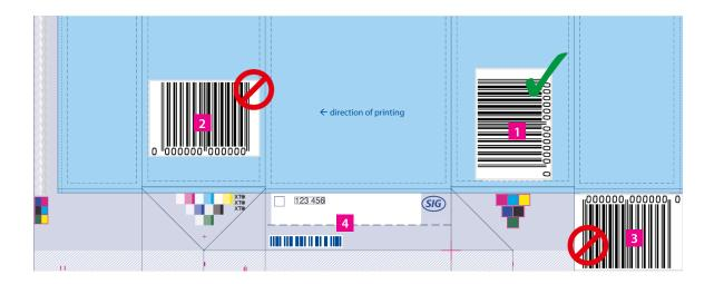
1 The code's standard position is parallel to the printing direction. SIG can only guarantee the readability of the code in the standard position and when the minimum code size is chosen.
