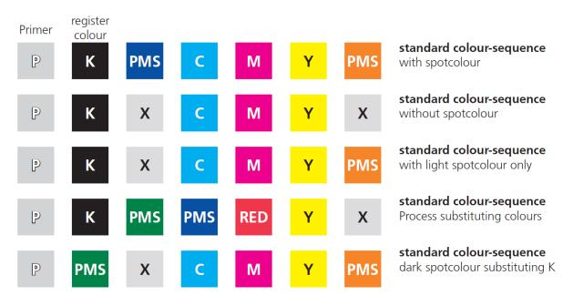
examples of standard color sequence for SIG SafeBloc (for bulk production)
